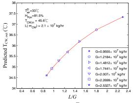
**Fig.6.** LMN predictions for  $T_{cw,out}$  vs. the water/air mass flow ratio.
