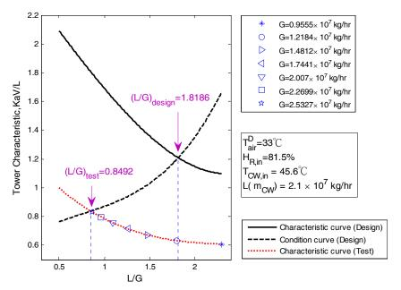
Fig.8. Tower characteristic vs. the water/air mass flow ratio.
