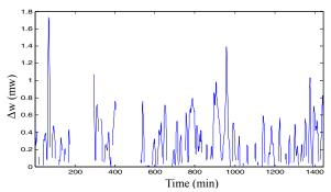
**Fig.5.** Total net power gain gain according to modified operating mode of fans.
