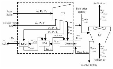
Fig.1. Process flow diagram of a typical PGS.
