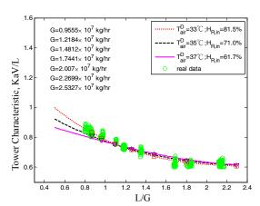
**Fig.7.** Predicted tower characteristic vs. calculated tower characteristic.
